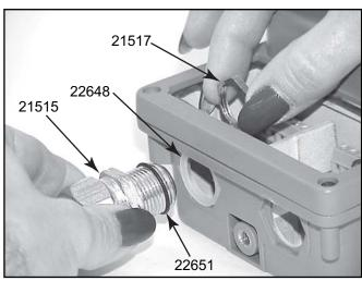
Insert 22648 in location as shown and then assemble 21515 with 21517. Roll 22651 back against hex nut before assembly.
